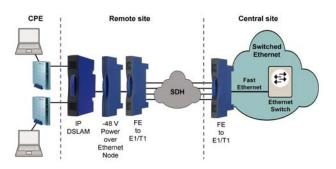
EXN104 supports up to four 120  $\Omega$  E1/T1 ports each with a speed of 2 Mbps. EXN104 conforms to ITU-T G.703 on the LSA® interface and is fully manageable via SNMP from PEM.
